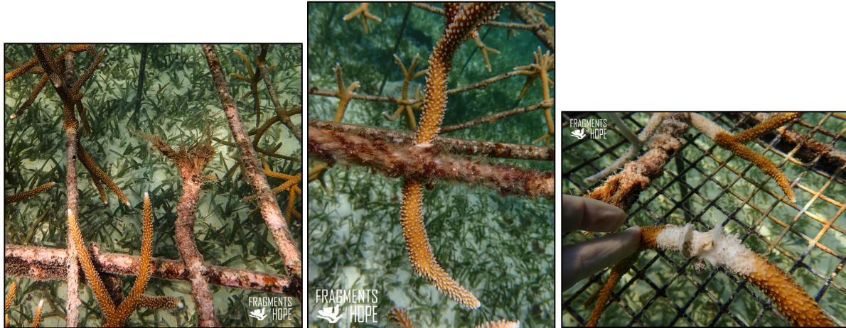
Figs. 7a-c. The hemp rope broke after ~eight months (L) and the corals could not grow over the hemp rope (center and right), as they usually do on the polypropylene ropes.
