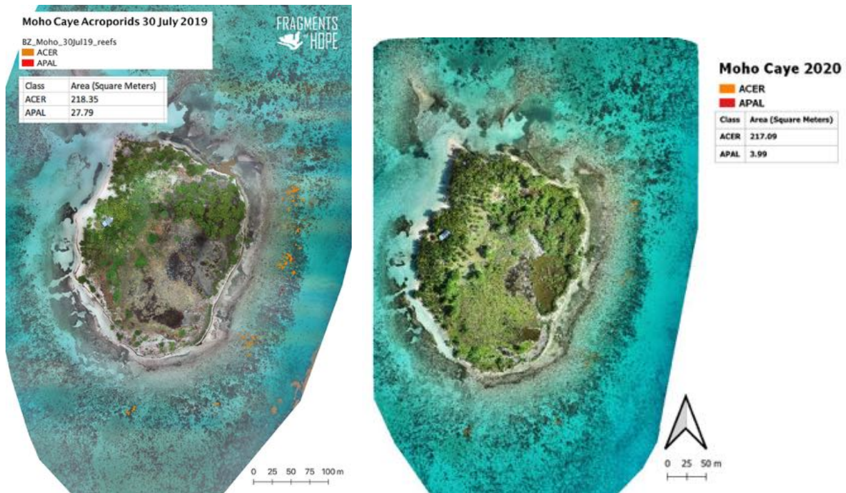
Fig. 17c-d. Object-based classification of coral features based on an orthophoto mosaic (2cm RGB) acquired with a DJI Phantom 4 Pro flying at 300ft on July 30, 2019 (L) and September 18, 2020 post-Nana. Here, the orange is replenished A. cervicornis and the red is natural/wild A. palmata .
